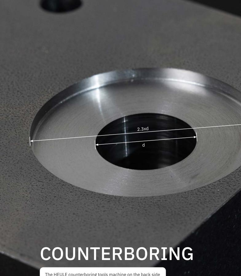
The HEULE counterboring tools machine on the back side of the bore without turning the workpiece. The counterbores are thus produced reliably on the machine without reclamping or manual intervention. The solutions are specially designed for fully automated production.
