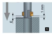
It is not necessary to change the sense of rotation nor to stop the spindle during the whole process. First, rapid traverse of the tool blade above the top material surface of bore or burr.
