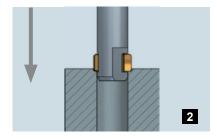
First, the burr of the front bore edge is being removed in working feed. Then, continue in working feed to apply the requested chamfer.
