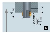
In back working feed the backward chamfer is executed. Proceed with the blade 1.0 mm farther than the planned chamfering depth.
