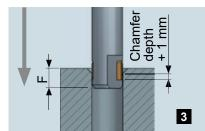
Continue in working feed 1.0 mm farther than the chamfer until the blade is fully retracted.
