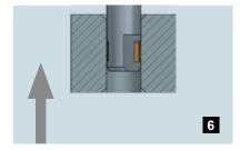
Once the blades are fully retracted, exit in rapid traverse to the next bore.
