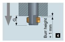
In rapid traverse and without stopping the spindle, you can travel through the hole without damaging its surface. Travel with the blade 1.0 mm behind the back bore edge and possible burrs.
