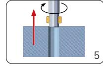
Rapid feed out of the workpiece
