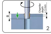
Working feed to position B or chamfer depth + 1.0 mm
