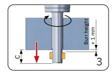
Rapid traverse to position C or burr height + 1.0 mm
