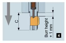
Go 1.0 mm beyond the existing burr in order to reach a safe initial position for the back chamfering.
