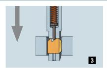
Rapid traverse through the hole. The surface of the hole cannot be damaged.
