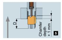
In back working feed the backward chamfering is executed. Proceed with the blade 1.0 mm farther than the planned chamfering depth.
