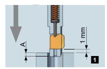
It is not necessary at all to change the sense of rotation or to stop the spindle during the whole process. First, rapid traverse of the tool blade above the top material surface of bore or burr.
