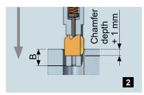
To generate the front chamfer continue in working feed until the blade is completely retracted into the tool.
