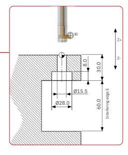
Cylindrical counterbore on the back of the bore
