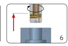
• Rapid feed out of the workpiece
