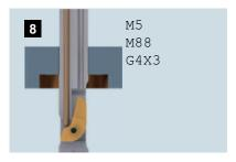
Spindle stop, internal coolant ON, 2-5 sec. dwell time (attention coolant pressure), blade retracts.
