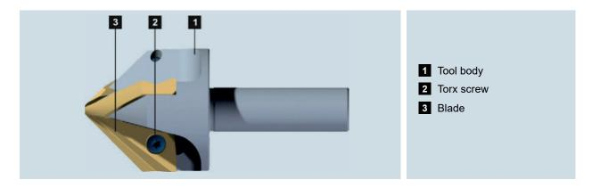
The toolbody made of alloyed heat treated steel together with the carbide blade enable the chatter-free production of countersinks on bores and chamfers on workpiece edges.
