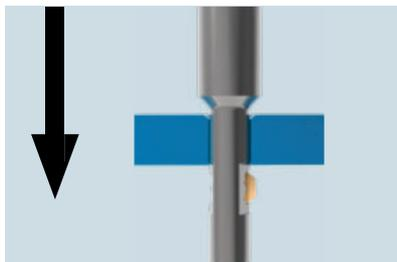
When it exits the bore, the SNAP blade is returned by the spring-loaded control bolt to the initial position.
