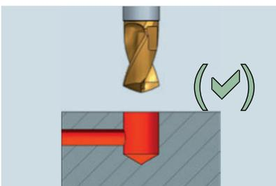
Drilling through a cross hole.  $\varnothing$  cross bore max 0.5xmain bore. If necessary, reduce feed rate<sup>2</sup>.
