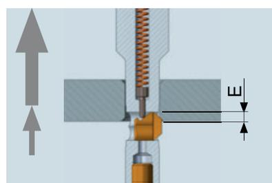
The back chamfer is machined by linear feed backward (no change of spindle direction). As soon as the SNAP blade is completely retracted into the tool, the tool can travel out of the hole in rapid feed backward.
