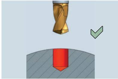
Drilling on central or convex surfaces<sup>1</sup>.
