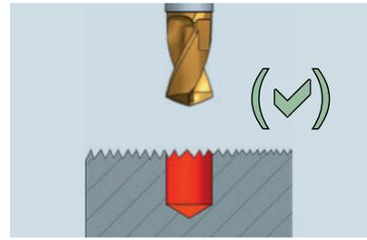
Drilling on uneven surfaces. If necessary reduce feed rate<sup>1</sup>.
