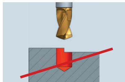
Drilling on an edge, forged or cast iron seam: Not possible.
