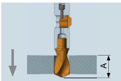
In forward linear feed the bore is produced. Continue in linear feed until the drill insert is completely clear of the bore.
