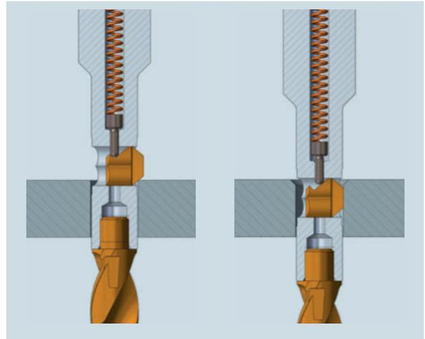
The SNAP chamfering blade is held by a spring-loaded control bolt in the tool body allowing it to move. The specially-ground SNAP blade for front and back or only back-cutting produces the required chamfer in **ONE OPERATION**. As soon as the defined chamfer thickness has been achieved, the SNAP radially enters the tool body. The chamfer thickness and angle are geometrically defined on the SNAP blade and can only be modified by inserting a different SNAP blade.
