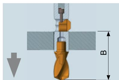
Position tool with SNAP blade in rapid feed, forward slightly above the top material surface of bore or burr.
