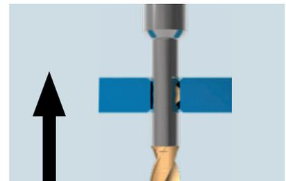
As soon as the back chamfer is completed, the tool can exit the workpiece in rapid traverse.
