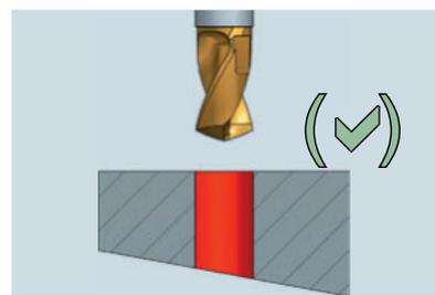
Sloped exit of the bore. Reduce feed rate to approx. 50-60%<sup>1</sup>.
