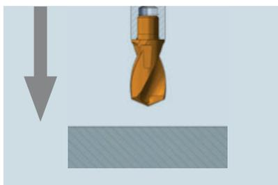
Rapid traverse of the tool to just above the top of the workpiece.
