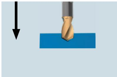
To do the drilling work, the tool is equipped with a screw-on high-performance helical drill bit.
