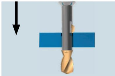
Drilling is followed by front and back chamfering using the integrated SNAP chamfering system. The specially ground SNAP blade for front and back or only back cutting produces the required chamfer.
