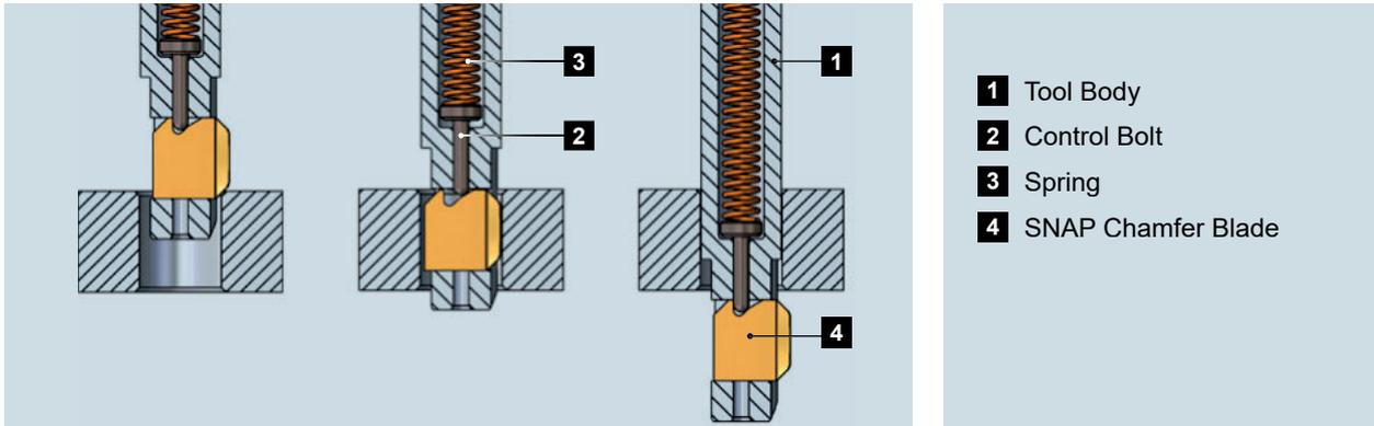
The SNAP deburring blade remains moveable in the tool body via a control bolt held under spring pressure. A specially ground forward and backward cutting only blade produces the required chamfer while the tool enters the bore. Once the chamfer size is attained, the deburring blade continuously retracts into the tool body. On a specially designed gliding radii, the blade passes through the hole without damaging it. The deburring
