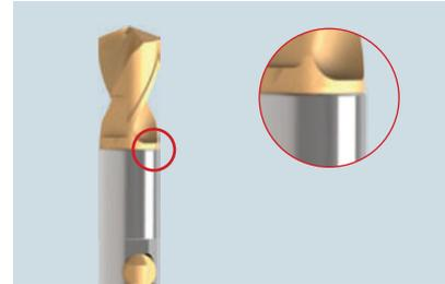
There should be a seamless transition between drill bit and tool body after the tightening of the drill bit (no light gap between tool body and drill bit).
