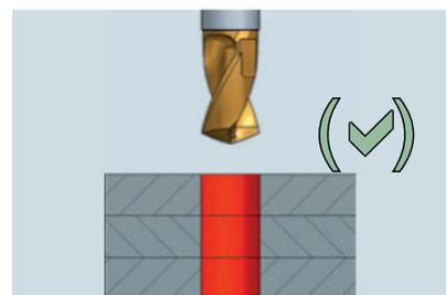
Drilling through several layers. Seamless clamping of the different workpieces is necessary.
