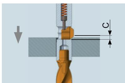
In linear feed forward, the chamfer is generated. Continue in linear feed until the blade is completely retracted into the tool.
