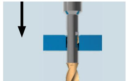
As soon as the defined chamfer thickness has been achieved, the SNAP radially enters the tool body.
