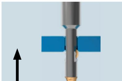
Without stopping the spindle or changing the sense of rotation, the tool produces the back chamfer on its way back.
