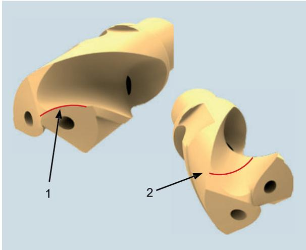
The patented VEX cutting geometry guarantees a high drilling performance with short chips. Due to the convex cutting edge (1), which merges into a concave chip angle (2) short chips are guaranteed even when machining long chipping material. A large chip channel also optimizes swarf evacuation.
