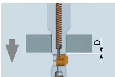
The tool can be passed through the hole in rapid feed forward until the SNAP blade is clear of the hole and fully extended.
