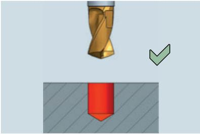
Drilling on even machined surfaces.
