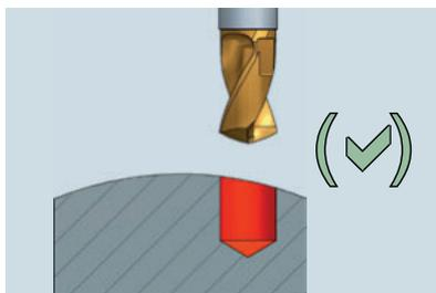
Drilling on not central or convex, concave surfaces<sup>1</sup>.
