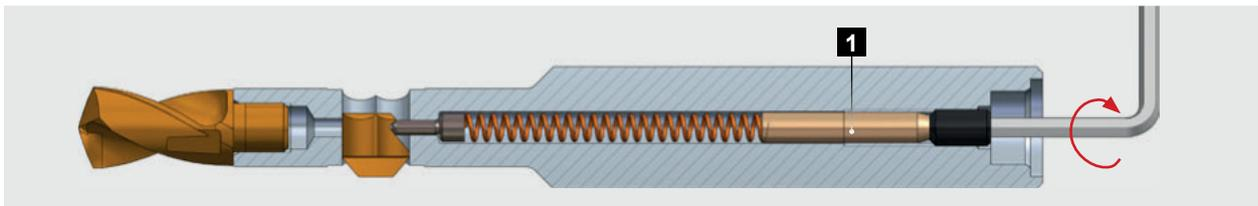
The blade force can be adjusted by the set screw (1) in the rear of the shank. The blade force has to be sufficient to extend the blade to fully after passing the back end of the bore. This ensures that the blade can work with the necessary cutting performance. The tougher the material, the tougher the spring should be set. The blade force, however, does not influence the chamfer size. Working with the correct blade pressure increases the blade life and improves the chamfer quality. An extremely
