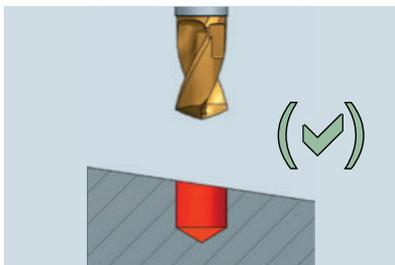
Drilling on sloped surfaces<sup>1</sup>.
