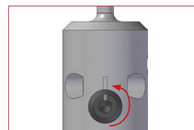
Turn back the excenter by 180° until the groove of the excenter is aligned with the groove in the tool body.
