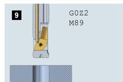
Now, move out of the workpiece in rapid speed.
