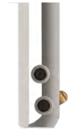
Neutral position of blade for forward machining
