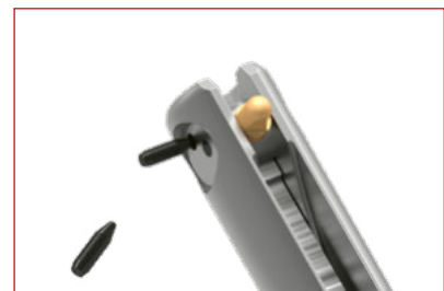
Loosen clamping screw and take the tool into your hands. Manually brake off the projecting section of the split pin at the predetermined breaking point.
