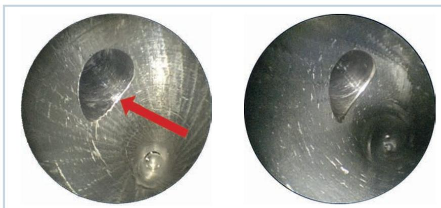
**3** An unprocessed borehole (left) and one processed with the COFA-X-based tool (arrow: burrs). The new tool removes burrs in a mechanically defined and therefore more reliable way (© Heule)
