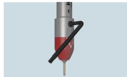
To complete the blade change, tighten the clamping screw using the Torx wrench.
